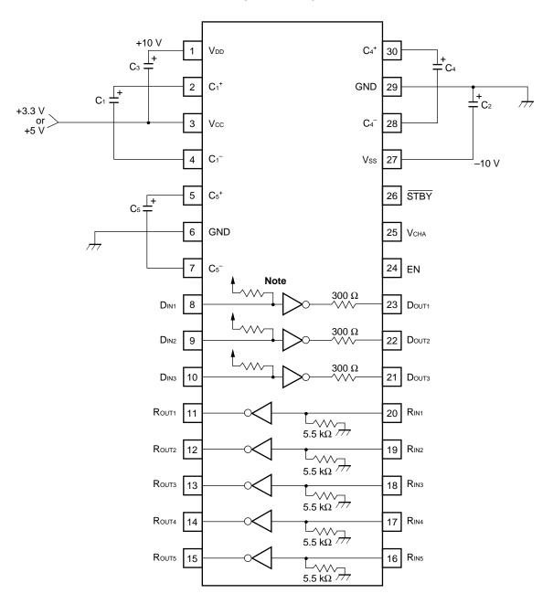
**Note** The pull-up resistors of the driver inputs are active resistors.
