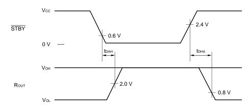
Receiver outputs are indefinite during transition time (tDHA).
